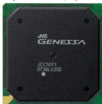
GENESSA “image intelligence” technology CPU-installed dedicated image processing LSI, integrated on a single system LSI.(sample)
